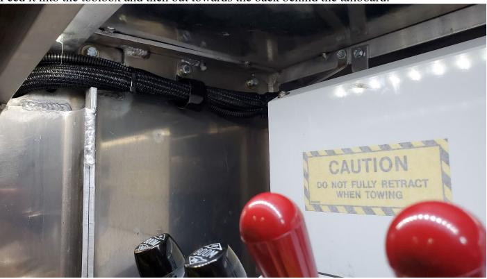
If no underlift rocker panels are to be installed, secure the connector using the dust cap above the connector such that moisture cannot collect around the sealed cap.
