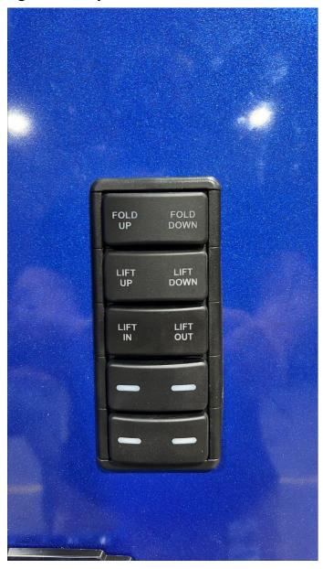
Install the part number 03013353 ROCKER ACTUATOR, LED -/- where the TILT was located on the tailboard control.
